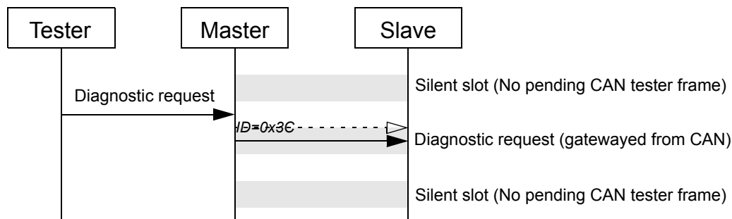
Figure 5.1: Gatewaying of CAN messages to LIN.
